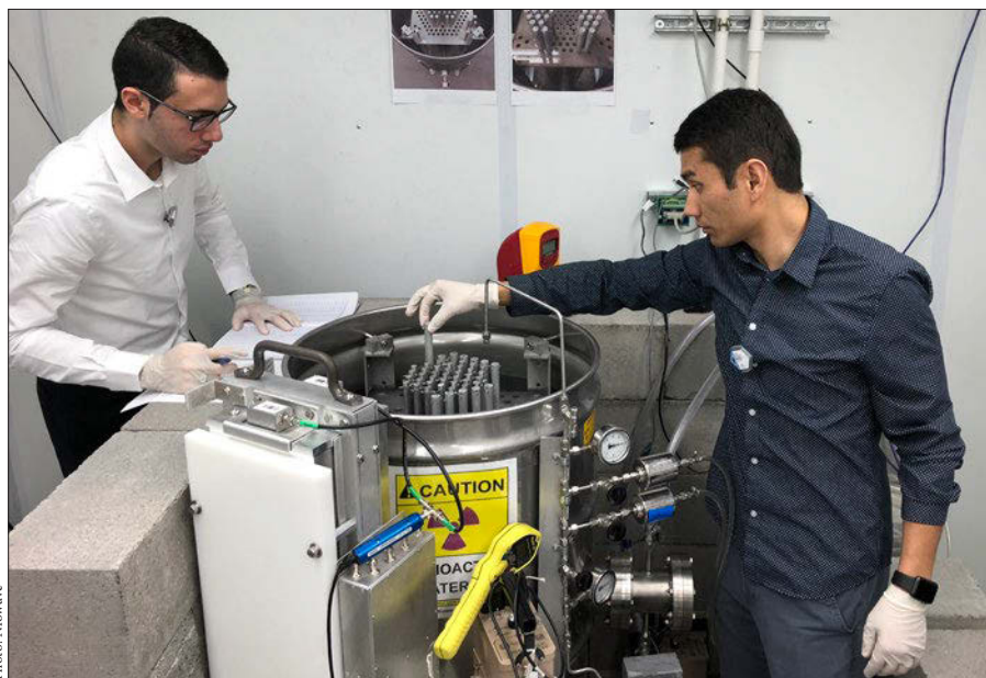
Two Niowave employees load a subcritical uranium target assembly for irradiation.
